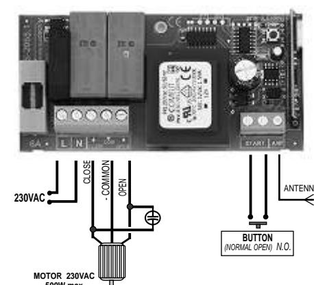
**MODEL S-2055** Control board for rolling shutters with built in limit switches and no needed photo cells
